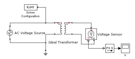
The next diagram would produce an error because it is lacking an electrical reference in the circuit of the secondary winding.
