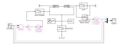
(highlighted in magenta). To avoid the algebraic loop, you can insert a Transfer Function block anywhere along the highlighted loop.
