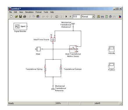
**10** Every time you connect a Simulink source or scope to a Simscape diagram, you have to use an appropriate converter block, to convert Simulink signals into physical signals and vice versa. Open the Simscape > Utilities library and copy a Simulink-PS Converter block and two PS-Simulink Converter blocks into the model. Connect the blocks as shown below.
