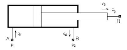
The element is represented with three energy flows: two flows of hydraulic energy through the inlet and outlet of the cylinder and a flow of mechanical energy associated with the rod motion. It therefore has the following three connector ports:
