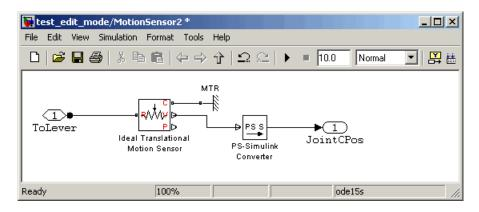
**4** Try to simulate the model. An error message appears saying that the model cannot be compiled because its topology has been changed while in Restricted mode. You can either undo the changes, or switch to Full mode, as described in "Switching from Restricted to Full Mode" on page 4-20.
