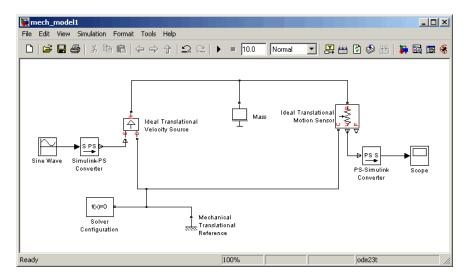
**Example.** The model shown in the following illustration contains an Ideal Translational Velocity Source directly connected to a Mass.
