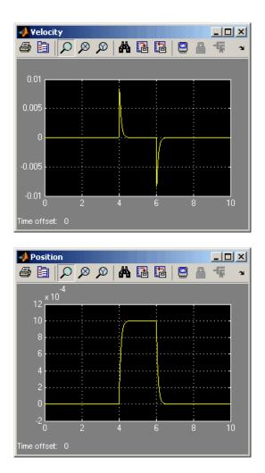
In the beginning, the mass is at rest. Then at 4 seconds, as the input signal changes abruptly, the mass velocity spikes in the positive direction and gradually returns to zero. The mass position at the same time changes more gradually, on account of inertia and damping, and stays at the new value as long as the force is acting upon it. At 6 seconds, when the input signal changes back to zero, the velocity gets a mirror spike, and the mass gradually returns to its initial position.
