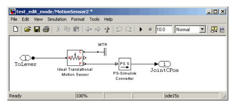
**3** Delete the connection line between port P of the Ideal Translational Motion Sensor block and the PS-Simulink Converter block. Instead, connect port V of the Ideal Translational Motion Sensor block to the input port of the PS-Simulink Converter block, to measure the velocity on node C of the lever.
