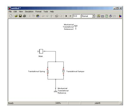
7 To add the representation of the force acting on the mass, open the Simscape > Foundation Library > Mechanical > Mechanical Sensors and Sources library and add the Ideal Force Source block to your diagram.
